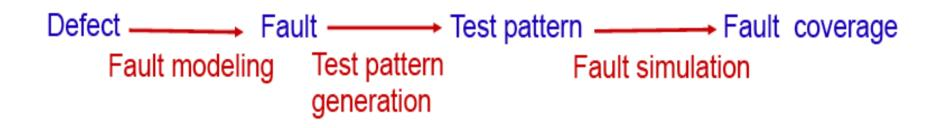
What faults to test (*fault modeling*)?
